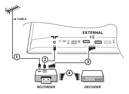
Note: Do not place your recorder too close to the screen as some recorders may be susceptible for signals from the display. Keep a minimum distance of 0,5 m from the screen.
