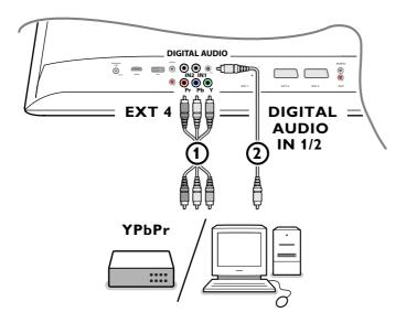
• Connect the three separate component video cables • to the peripheral equipment having component video outputs (YPbPr), such as DVD-players, laser-disc players, videogame players, satellite receivers or other equipment, and to the **Y**, **Pb** and **Pr** jacks of **EXT4** on the TV.
