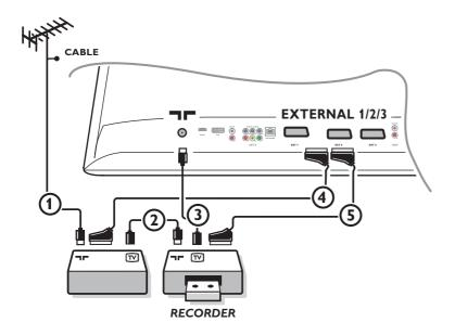
Connect the aerial cables ①, ② and ③ as shown (only if your peripheral has TV aerial in-/output).
