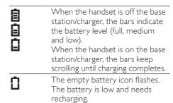
The handset turns off if the batteries are empty. If you are on the phone, you hear warning tones when the batteries are almost empty. The call gets disconnected after the warning.
