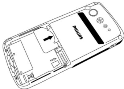
Place the battery back into its slot, with the gold contacts of the battery facing the corresponding gold contacts on the side of the phone. The gold contacts on the phone are positioned on the right hand side of the phone, besides the SIM card slot.
