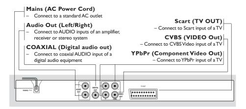
Caution: Do not touch the inner pins of the jacks on the rear panel. Electrostatic discharge may cause permanent damage to the unit.
