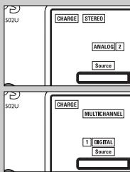
**7** The signal format (stereo/ multichannel) will be analyzed automatically and indicated on the display panel:
