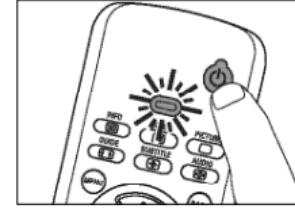
**4** When your TV switches off (stand-by), release the Standby key of the SRU 5010 immediately.
