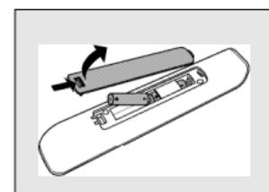
Note: If the LED blinks four times after every key press, the remote control is indicating that its batteries are running low. Replace the old batteries with two new AAA batteries.
