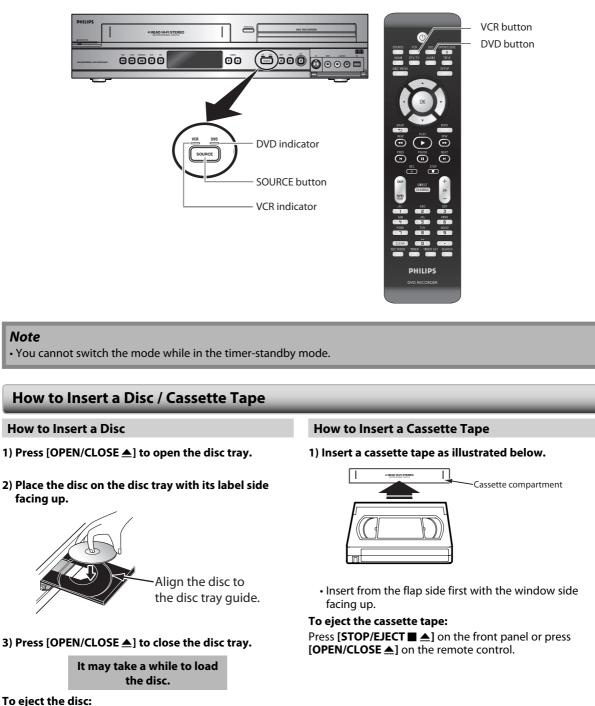
Press [**OPEN/CLOSE**  $\triangleq$ ] to open the disc tray, then remove the disc before turning off the unit.
