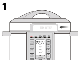
1 Secure and lock lid in a clockwise direction by aligning arrows.
