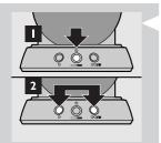
5 Press the on/off button 𝒪 (1) and subsequently press buttons the 1-cup button 𝒪 and the 2-cup button 𝑃𝒪/➡ briefly at the same time (2).
