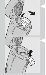
Take the coffee spout out of the machine by sliding it upwards. The coffee spout can only be taken out after the coffee collector has been removed.
