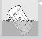
8 Clean the water reservoir in hot water, if necessary with some dish soap.
